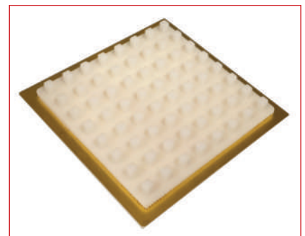
▲ Fig. 4 Three-dimensional view of an 8×8 array of uniformly spaced DRA elements.
